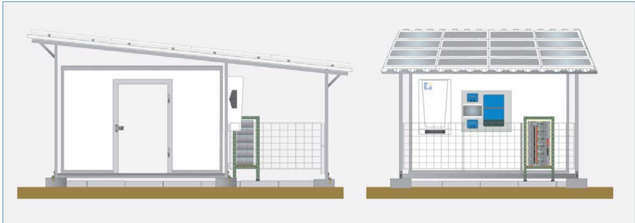
Figure 23. AC cooling unit with Li-ion battery bank and controller/inverter unit. (Source [35])
