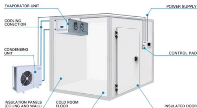
Figure 1. Main components of a cold room. (Source[9]).
